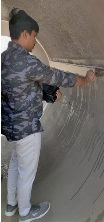
Madhu performs quality control using an ultrasonic device to find discontinuities under the welds and to help check pipe quality.
